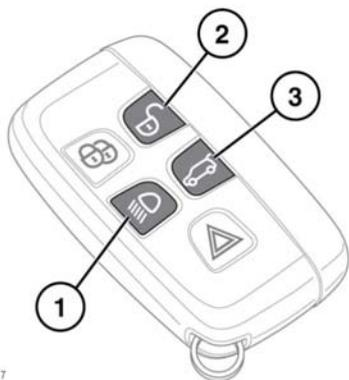
To raise the vehicle, press and hold the approach lamps button (1) and the unlock button (2) together.
