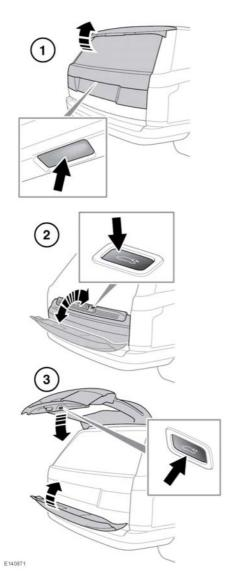
1. Upper tailgate open/close using the exterior button. Press to open, stop, reverse direction or close the upper tailgate. Press to close the upper and lower tailgates.
