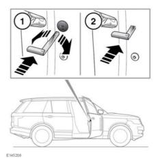
In the event of the battery discharging or a fault with the Keyless locking system, each door must be locked manually.
