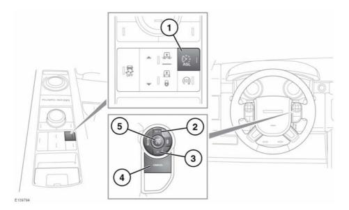
ASL allows a speed limit to be set that the driver does not wish to exceed.
