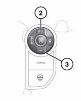
If HDC is deselected while operating, the lamp will flash and the system will fade out, allowing the vehicle's speed to gradually increase.
