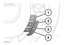
SET+: Press to set the speed or to increase the set speed. The cruise control warning lamp will illuminate to confirm cruise control is operational. See 49, CRUISE CONTROL (GREEN).
