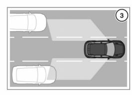
The Blind Spot Monitor (BSM) system monitors a zone that covers the area adjacent to the vehicle, that is not easily visible by the driver and is designed to identify any object overtaking the vehicle (3). The system uses a radar on each side of the vehicle to identify any overtaking vehicle/object within the blind spot area of the vehicle, while disregarding other objects which may be stationary or travelling in the opposite direction. etc.
