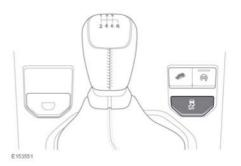
To disable DSC, press and briefly hold the DSC OFF switch. The DSC OFF warning lamp will illuminate. See **98**, **DYNAMIC STABILITY CONTROL (DSC)**. Deactivating DSC also reduces the level of Electronic Traction Control (ETC) intervention and may lead to an increase in wheel spin.
