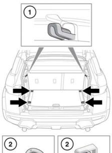
2. Load securing lashing eyes: To assist in safely securing large items of luggage, 4 lashing eyes are located in the rear loadspace floor.
