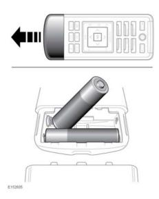
Low battery power is indicated by the remote control power button flashing 3 times when pressed. To renew the batteries:
