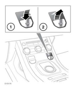
With the ignition turned on, depress the brake pedal, then press down and release the EPB switch. This will release the EPB. With the vehicle stationary, pull up and release the EPB switch. This will apply the EPB. The parking brake warning lamp will illuminate to indicate that the parking brake is applied. See 46, PARKING BRAKE (RED).
