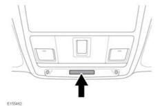
An airbag status indicator, mounted on the overhead control panel (as illustrated), will display the operational status of the passenger airbag.
