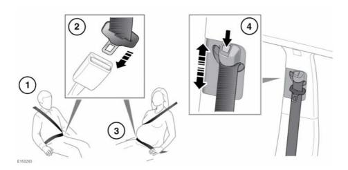
Putting on a seat belt: Draw the belt out smoothly, make sure the belt height, the seat and your position on the seat, are correct.
