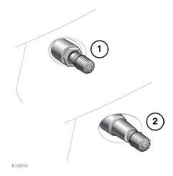
Wheels fitted with TPMS can be visually identified by the external metal lock nut and valve (1). All Land Rover non-TPMS wheels have a rubber valve fitted (2).
