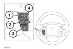
SET+: Press to set the speed or to increase the set speed. The Cruise control warning lamp will illuminate to confirm that Cruise control is operational. See 37, CRUISE CONTROL (GREEN).
