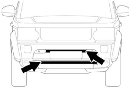
Using a hose pipe, direct clean water through the front bumper (where shown), to remove mud on the radiator and air conditioning condenser.
