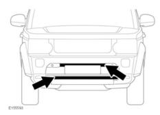
Using a hose pipe, direct clean water through the front bumper (where shown), to remove mud on the radiator and air conditioning condenser.
