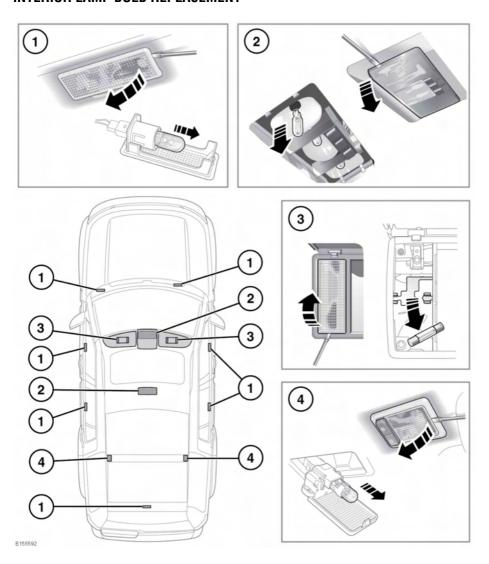
Follow the steps illustrated. Insert a new bulb and refit the components.
