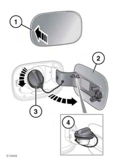
The fuel filler flap is located on the right side of the vehicle, at the rear.
