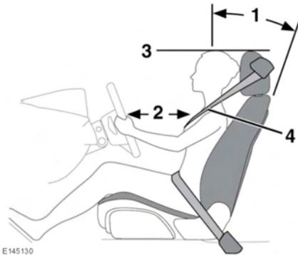
**⚠ The driver and front seat passenger must not ride with the seat fully reclined.**
