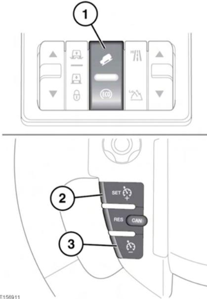
Hill Descent Control (HDC) is designed to restrict vehicle speed to a set limit when travelling downhill.
