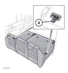
Pull the strap (4) vertically to unlock the seats, then raise the seats by following the lowering process in reverse.
