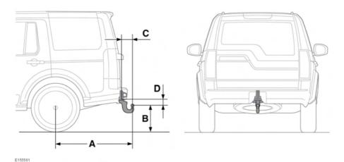
Ref. Dimension Metric **Imperial** Wheel centre to centre of tow ball 1.190 mm Α 46.9 in. Ground to centre of tow ball 16.1 in. В 409 mm Centre of tow ball to tow bar 6.7 in. C 170 mm attachment D Centre of tow ball to tow bar 124 mm 4.9 in. attachment
