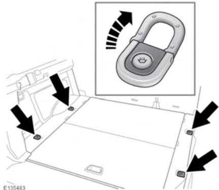
To assist in safely securing large items of luggage, 4 fixing points are located in the rear loadspace floor.
