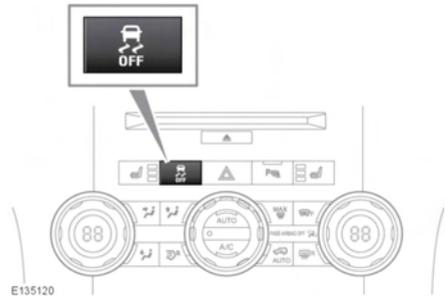
To disable DSC, press and briefly hold the **DSC OFF** (arrowed) switch on the fascia (the DSC off warning lamp will illuminate continuously). Deactivating DSC also reduces the level of Traction control intervention and may lead to an increase in wheel spin.
