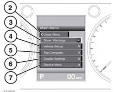
A number of vehicle features and display settings may be configured via the Instrument panel menu.
