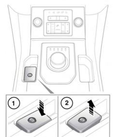
The switch which operates the EPB is mounted on the centre console, to the side of the gear selector.
