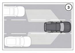
The Blind Spot Monitor (BSM) system monitors an area adjacent to your vehicle, that is not easily visible to the driver. The system is designed to identify any road user overtaking your vehicle (3) that is within this blind spot, while disregarding other objects which may be stationary or travelling in the opposite direction.
