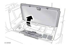
**5 seat vehicles**: The tool kit is located under a panel set in the loadspace floor.
