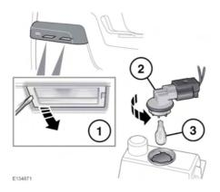
Follow the steps illustrated. Insert a new bulb and refit the components.
