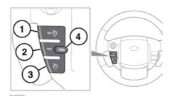
SET+: Press to set the speed or to increase the set speed. The Cruise control warning lamp will illuminate to confirm Cruise control is operational (see 46, CRUISE CONTROL (GREEN)).
