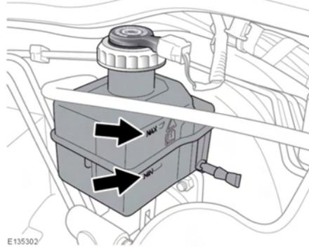
The left side or right side under bonnet cover must be removed to check the brake fluid level, dependent on the vehicle being left hand drive (left side cover) or right hand drive. See **194, UNDER BONNET COVERS - REMOVAL**.
