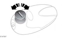
With the back of the remote control facing upwards, use a coin or a similar implement to rotate the battery cover. Lift the cover off, to reveal the battery compartment. Remove the old battery, and making sure that the correct polarity is maintained, insert a replacement 3.3-volt, CR1/3N battery. Replace the cover and rotate it to lock closed.
