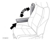
If fitted, the folding armrest may be stowed by moving to the vertical position. Use the adjuster wheel (arrowed) to set the required height.
