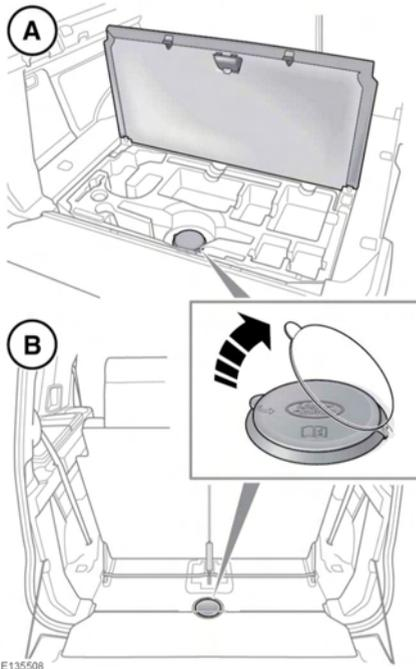
**⚠** Remove the spare wheel prior to jacking the vehicle, to avoid destabilising the vehicle, when raised.
