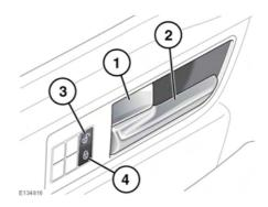
From inside the vehicle, all of the doors can be locked by pressing either the driver or passenger lock lever (1).
