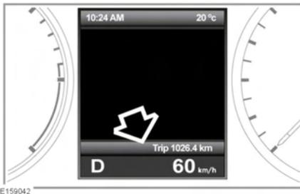
A short press (1 second or less), or a series of short presses of the **i** button (arrowed), will change the Trip computer display.
