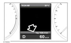
A short press (1 second or less), or a series of short presses of the i button (arrowed), will change the Trip computer display.
