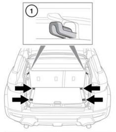
2. Load securing lashing eyes: To assist in safely securing large items of luggage, 4 lashing eyes are located in the rear loadspace floor. If adjustable lashing eyes are fitted, first turn the locking button counter clockwise to unlock. Press the button and slide to the required position in the luggage rail. Release the button to latch into position. Move the lashing eye slightly until you hear a click.
