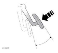
Clutch pedal travel is set at the factory and is non-adjustable.
