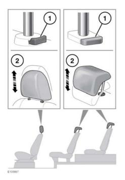
If removal is essential, move the head restraint to its highest position then squeeze in the locking collar while lifting the restraint clear of the seat.
