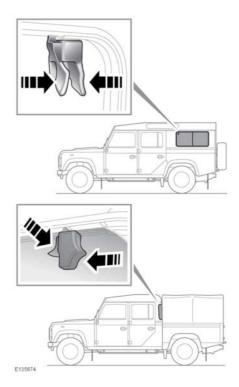
Squeeze either type of lock and slide the window to the desired position. Release the lock and make sure that the catch is located securely into a locking socket.
