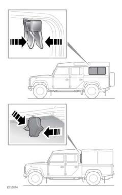
Squeeze either type of lock and slide the window to the desired position. Release the lock and make sure that the catch is located securely into a locking socket.
