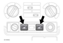
**Note:** To prevent the battery from becoming discharged, the seat heaters should be operated only when the engine is running.
