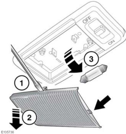
1. Insert a small flat bladed screwdriver into the indent at the side of the lens.
