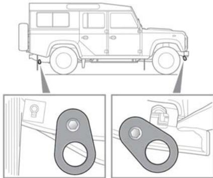
**⚠** The towing eyes at the front and rear of the vehicle are designed for on-road recovery only. If they are used for any other purpose it may result in vehicle damage and serious injury.
