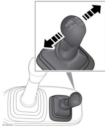
**Locking the differential:** With the transfer box in either High or Low range, press the clutch and move the lever to the left. When the lock is engaged, a warning lamp will illuminate in the Instrument panel.
