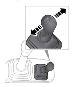
Locking the differential: With the transfer box in either High or Low range, press the clutch and move the lever to the left. When the lock is engaged, a warning lamp will illuminate in the Instrument panel.
