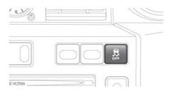
To disable DSC, press and briefly hold the DSC OFF button. The DSC OFF warning lamp will illuminate. See **30**, **DYNAMIC STABILITY CONTROL (DSC) OFF (AMBER)**. Deactivating DSC also reduces the level of Electronic Traction Control (ETC) intervention and may lead to an increase in wheel spin.
