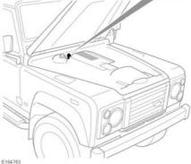
The fuel cut-off switch is a safety device which, in the event of a collision or sudden impact, automatically cuts off fuel supply to the engine.
