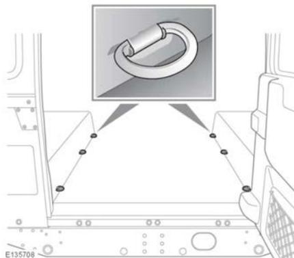
On some vehicles, load securing rings are provided in the rear of the vehicle to assist in safely securing luggage.
