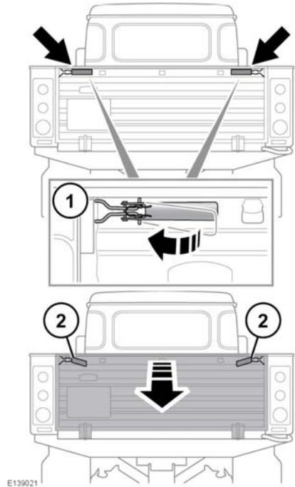
1. Lever the latches outwards, toward the sides of the vehicle.
