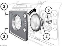
In order to change a headlamp unit bulb, you must first remove the headlamp unit:
