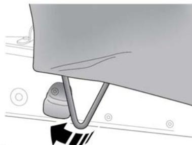
Starting at the front of the canopy, loop the tie rope over each of the hooks along the sides of the vehicle. Make sure that each loop is tightened before the next loop is made.
