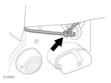
Fasten the rope to the hook above the rear lamps.
