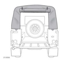
Roll up the rear screen and secure with the straps.
