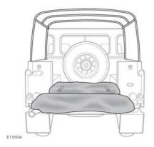
With the roof frame in position, lay the canopy on the open tailgate.
