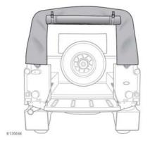
Roll up the rear screen and secure with the straps.
