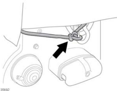
Fasten the rope to the hook above the rear lamps.
