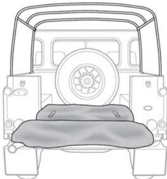
With the roof frame in position, lay the canopy on the open tailgate.
