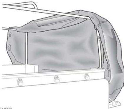
From the rear, lift the canopy over the frame, making sure that the front window is against the cab window.
