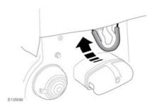
Pull and attach both rubber hoops to the hooks, above the rear lamps.
