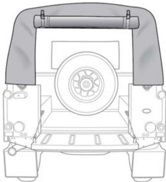
Roll up the rear screen and secure with the straps.
