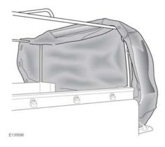
From the rear, lift the canopy over the frame, making sure that the front window is against the cab window.
