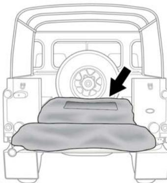
Unfold the canopy into the load area.
