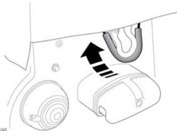
Pull and attach both rubber hoops to the hooks, above the rear lamps.
